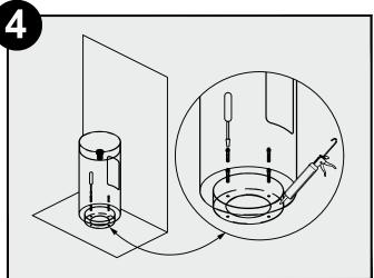
Apply a clear silicone to the base of the sink. Place it back in the correct position and fasten the screws.
