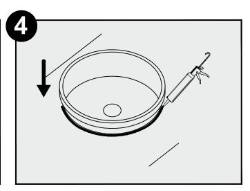
Clean and dry the surface around the opening of the sink. Verify that the sink fits correctly in the opening. The edge of the sink must sit on the counter. Apply silicone-based sealant (not included) underneath the edge of the sink rim. Lower the sink into position. Place a weight in the sink for 24 hours while the silicone cures.
