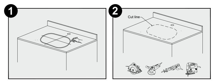
Use the template provided or the DXF file to create the cutout in the countertop. It is recommended to have a 1/8" to 1/4" overhang.
