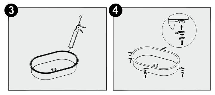
Clean and dry the surface around the opening of the sink. Check the alignment of the sink to the opening in the countertop. Apply silicone-based sealant (not included) around the rim of the sink. Place the sink over the cutout hole and press firmly. Use your own preferred clamping system to secure the sink to the underside of the countertop opening. Make sure it is accurately aligned to the cutout opening.
