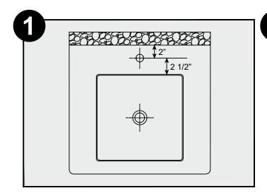
Place the sink in the desired location on the countertop and mark the drain hole and faucet hole centerline with a pencil.
