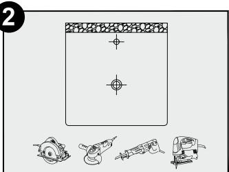
Drill the drain and faucet holes with the suitable tools according to the countertop material.
