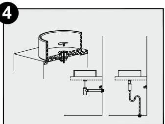
Apply clear silicone around the bottom of the sink and place it over the drain hole.
