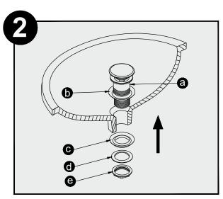
Install the drain body (a), with the thin gasket (b) attached, into the drain hole of the vanity bowl. From underneath the bowl, attach concave washer (c) (narrow end facing up), plastic washer (d) and mounting nut (e) to the drain body (a).
