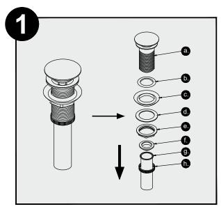
Begin by removing the nut (h), tailpiece (g), mounting nut (e), plastic washer (d) and concave washer (c) from the drain body (a).
