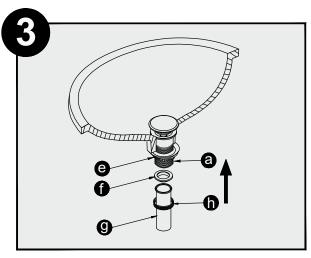
Tighten the mounting nut (e) with an adjustable wrench until snug. Thread the nut (h) with the tailpipe (g) attached, onto the drain body (a) and hand tighten.
