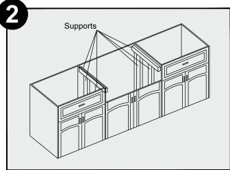
Measure the thickness of the sink's side rims. They are approximately 3/8" thick. Position horizontal wood support strips this measured distance below the top of the side walls of the cabinet. Screw in securely. Place vertical support strips between floor of the cabinet and the horizontal support strips to provide additional support.
