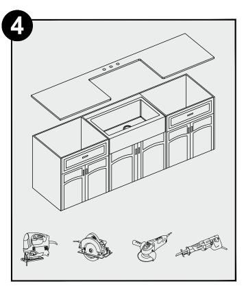
Template the sink and countertop for fabrication once the sink is installed in the sink base cabinet. Cut the opening in the countertop based on the sinks actual measurements.
