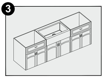
Place the sink in the opening. The weight of sink should be sustained by the built supports. Make sure sink is level from front to back and side to side. Ensure the top surface of the sink rim is flush with the tops of the cabinet walls. Position the sink so that the sides of the apron are recessed into the face frame of the cabinet by approximately 3/4".
