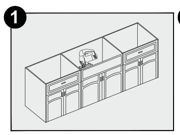
Measure the width and height of the apron front. Add 1/16" to these dimensions. Tape off the face of the cabinet with painters tape then mark the face of the cabinet with this cutout size. This cutout should be flush to the top of the face frame and centered left to right. Carefully make the cutout using a jigsaw. Sand the edges of the cutout to ensure they are clean and straight.
