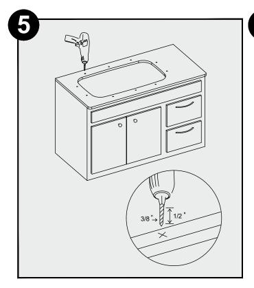
Drill 3/8" diameter x 1/2" deep hole in the countertop. Loosely install the fasteners.
