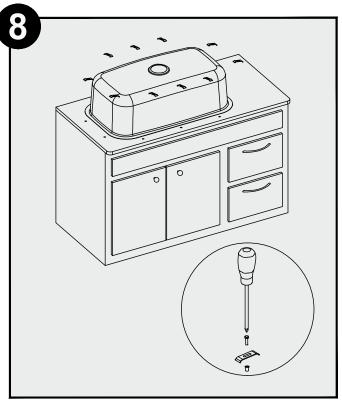
Attach mounting hardware to secure bowl. Remove excess sealant from inside lip. Allow sealant to set for 30 - 60 minutes.
